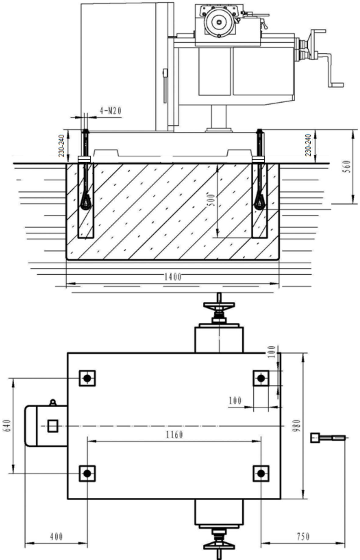
DIAGRAM 3 MACHINE FOUNDATION
