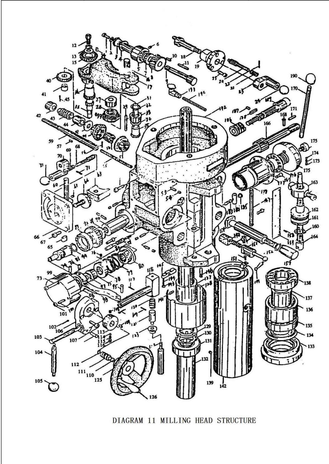
DIAGRAM 11 MILLING HEAD STRUCTURE
