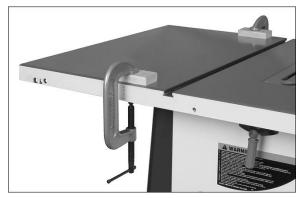
Figure 5-6: leveling extension wings, method 2
