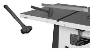
Figure 5-5: leveling extension wings, method
